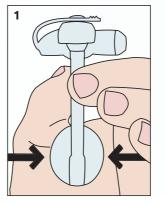
Take the 10 ml Luer syringe from the danuButton® set and fill the balloon with sterile water via the balloon valve.
